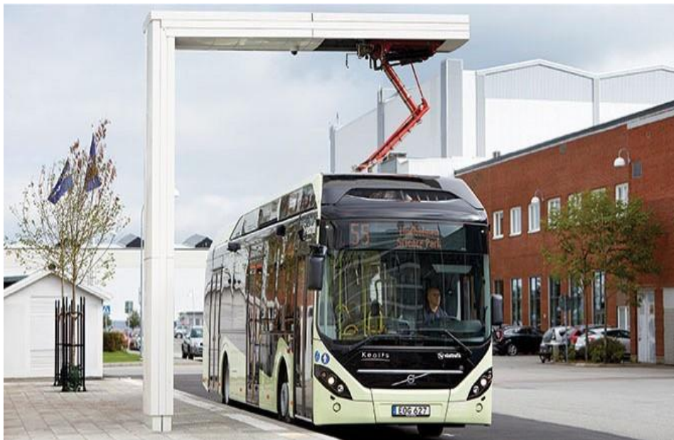
Figure 6.20: Electric Vehicle Charging Station for Buses
